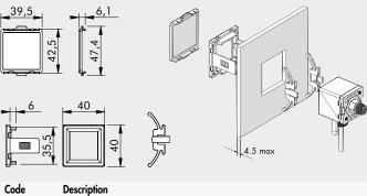
9000643 Kit for panel fixing with protection for the digital pressure switch series 640
