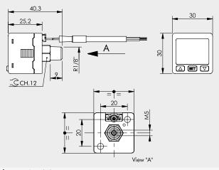
Code Description 9000640L Digital pressure switch series 640 IO-Link
