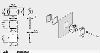
Description 9000643L Kit for panel fixing with protection for the digital pressure switch series 640 IO-Link **C6**
