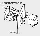
Code Description 9000603 Kit for panel fixing with protection for the digital pressure switch series 600
