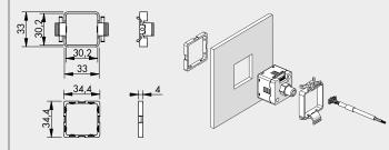
Code Description 9000642L Kit for panel fixing for the digital pressure switch series 640 IO-Link
